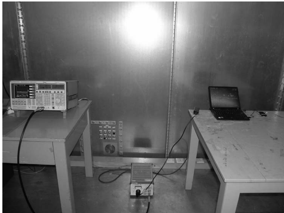
Photograph 1: Set-up for Conducted Emission Measurement
