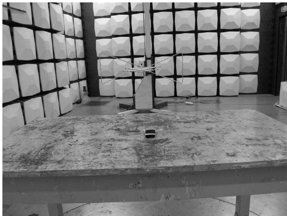
Photograph 2: Set-up for Radiation Measurement below 1GHz
