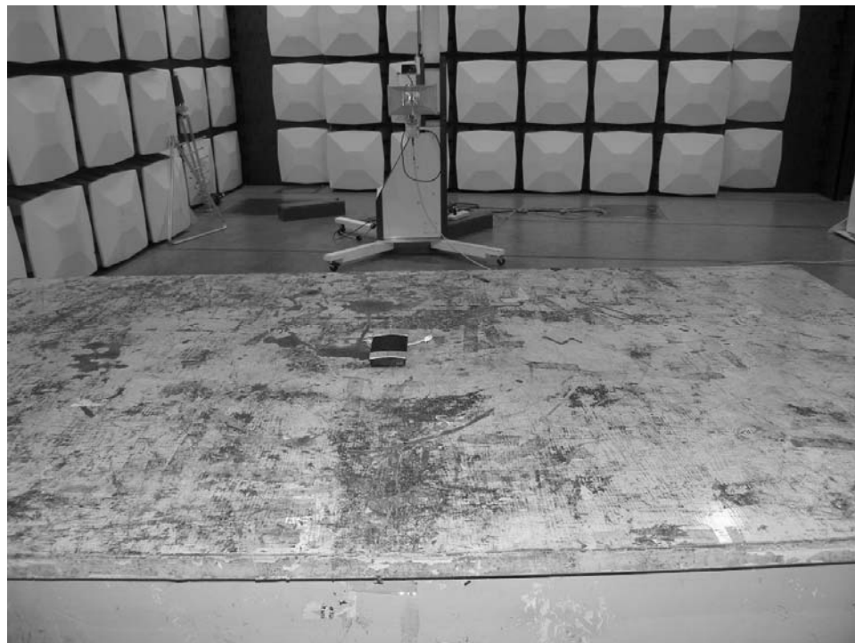
Photograph 3: Set-up for Radiation Measurement above 1GHz
