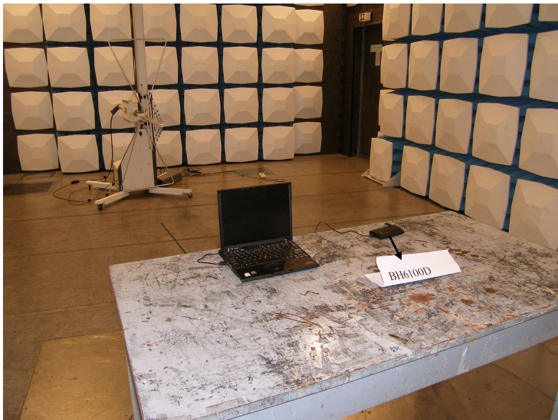
Photograph 2: Set-up for Radiation Measurement below 1GHz
