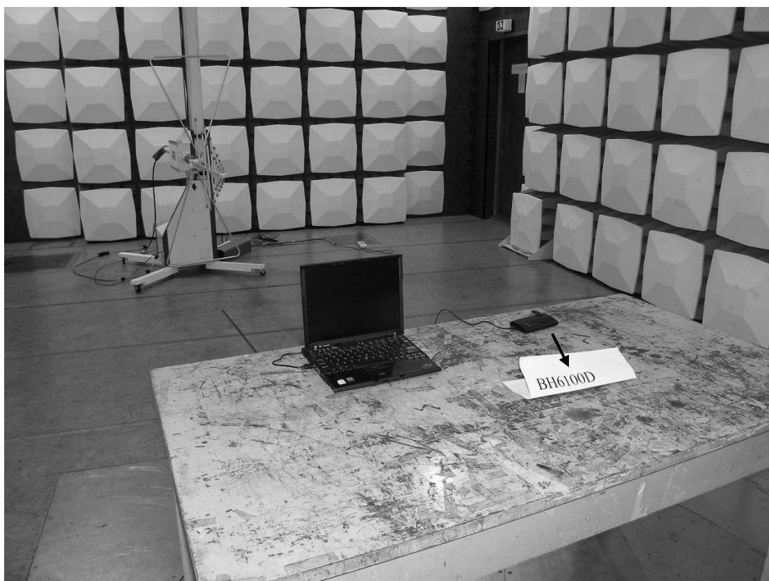
Photograph 2: Set-up for Radiation Measurement below 1GHz
