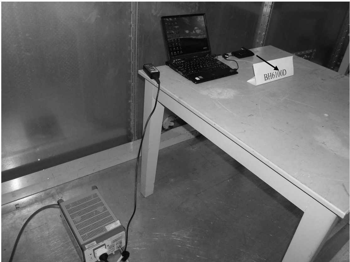
Photograph 1: Set-up for Conducted Emission Measurement
