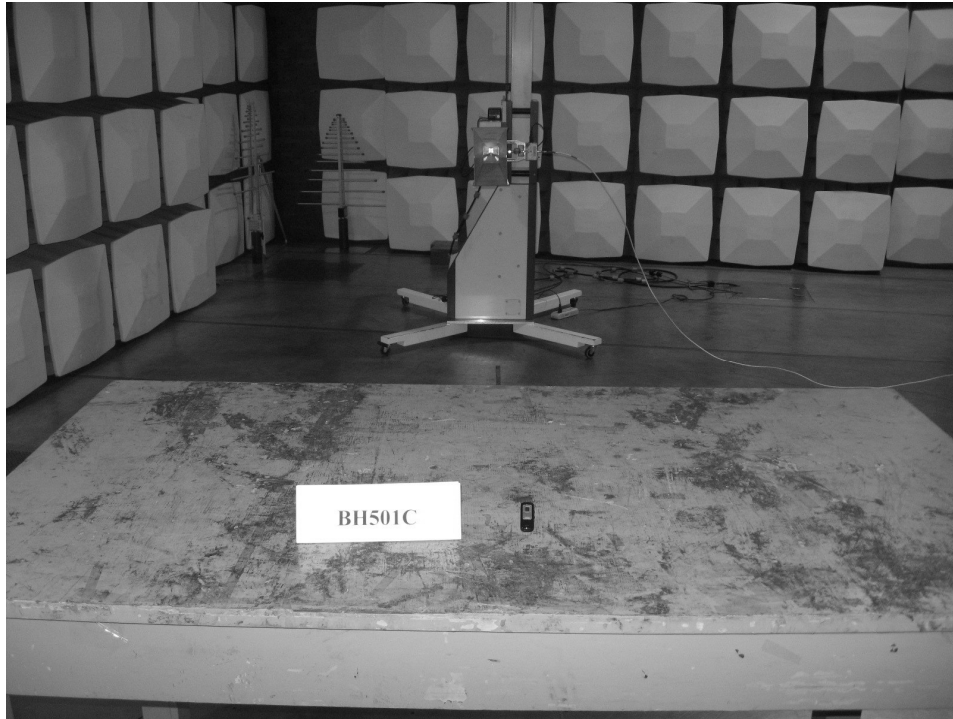
Photograph 3: Set-up for Radiation Measurement above 1GHz
