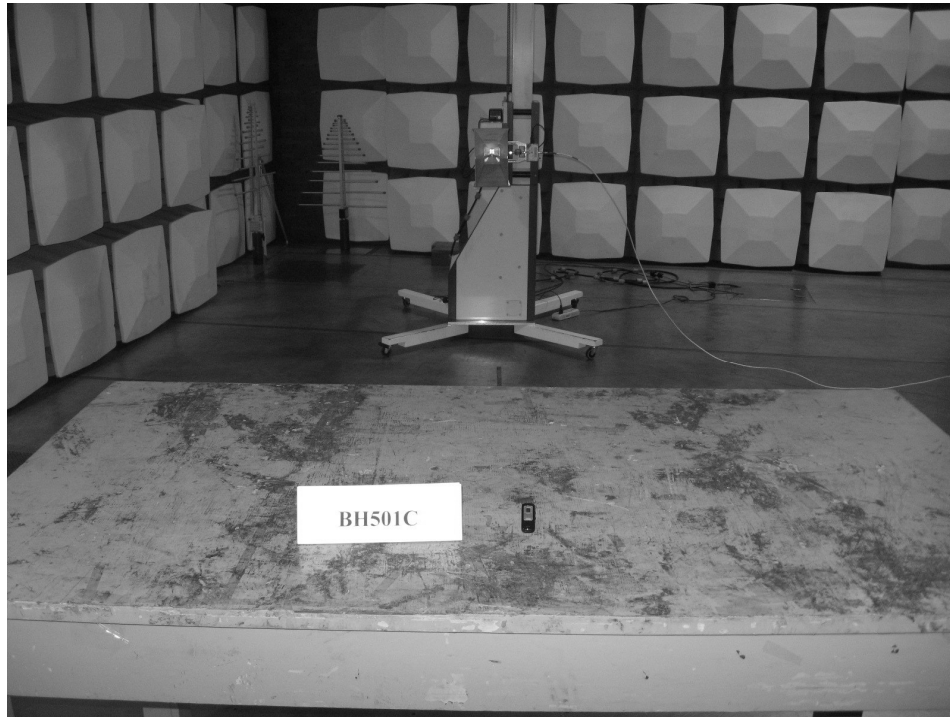
Photograph 3: Set-up for Radiation Measurement above 1GHz
