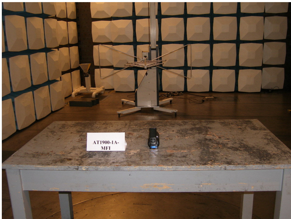
Photograph 2: Set-up for Out of band emissions (30MHz-1GHz)
