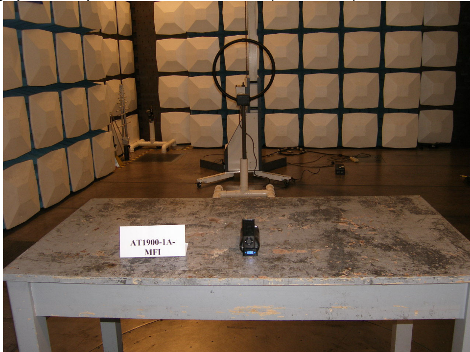
Photograph 2: Set-up for Out of band emissions (30MHz-1GHz)
