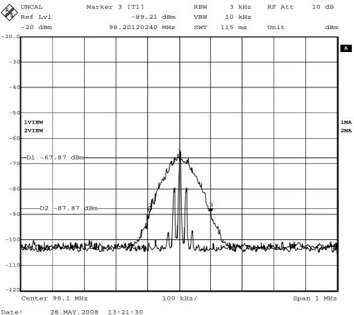
Low Frequency is 98.0068 MHz, High Frequency is 98.2012MHz
