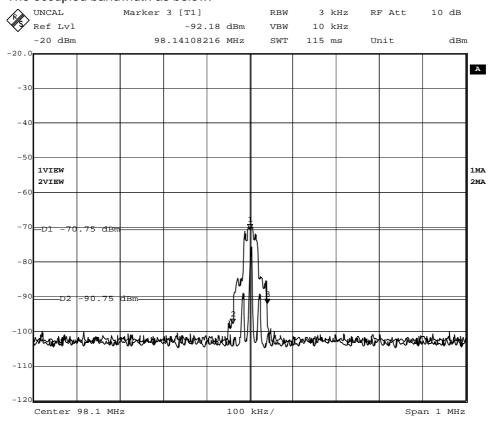
Low Frequency is 98.0609MHz, High Frequency is 98.1411MHz
