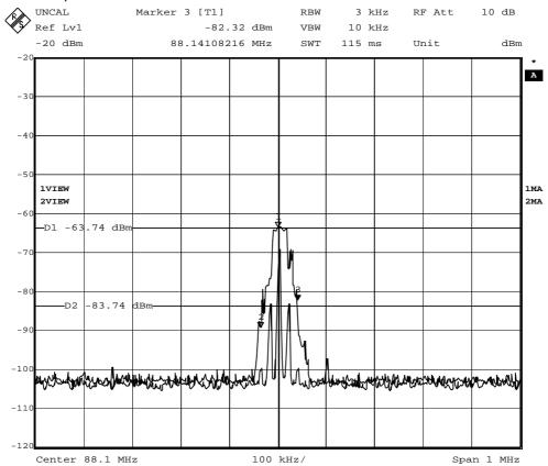
Low Frequency is 88.0649MHz, High Frequency is 88.1410MHz
