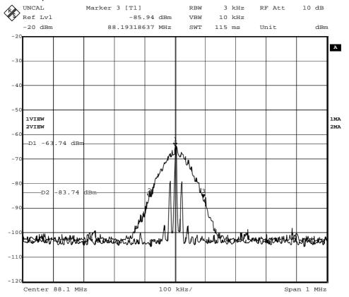
Low Frequency is 88.0120 MHz, High Frequency is 88.1932MHz
