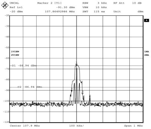
Low Frequency is 107.8709 MHz, High Frequency is 107.9471MHz
