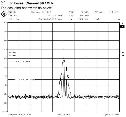
Low Frequency is 88.0649MHz, High Frequency is 88.1410MHz
