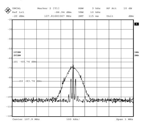
Low Frequency is 107.8168 MHz, High Frequency is 107.9871MHz
