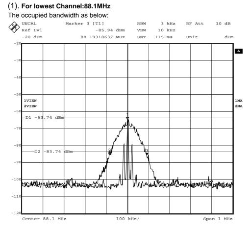
Low Frequency is 88.0120 MHz, High Frequency is 88.1932MHz
