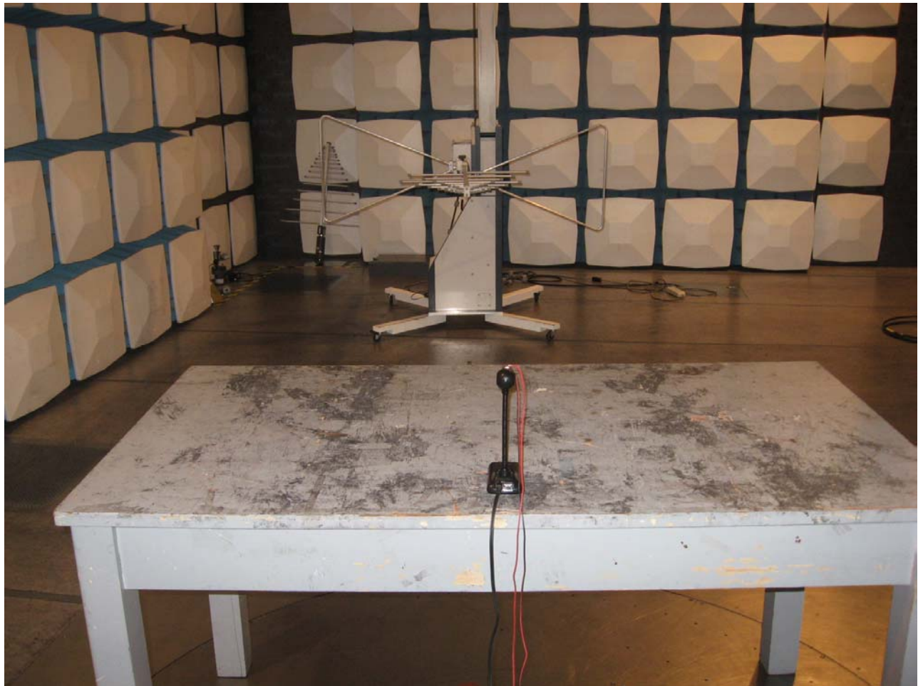
Photograph 1: Set-up for Radiated Emission
