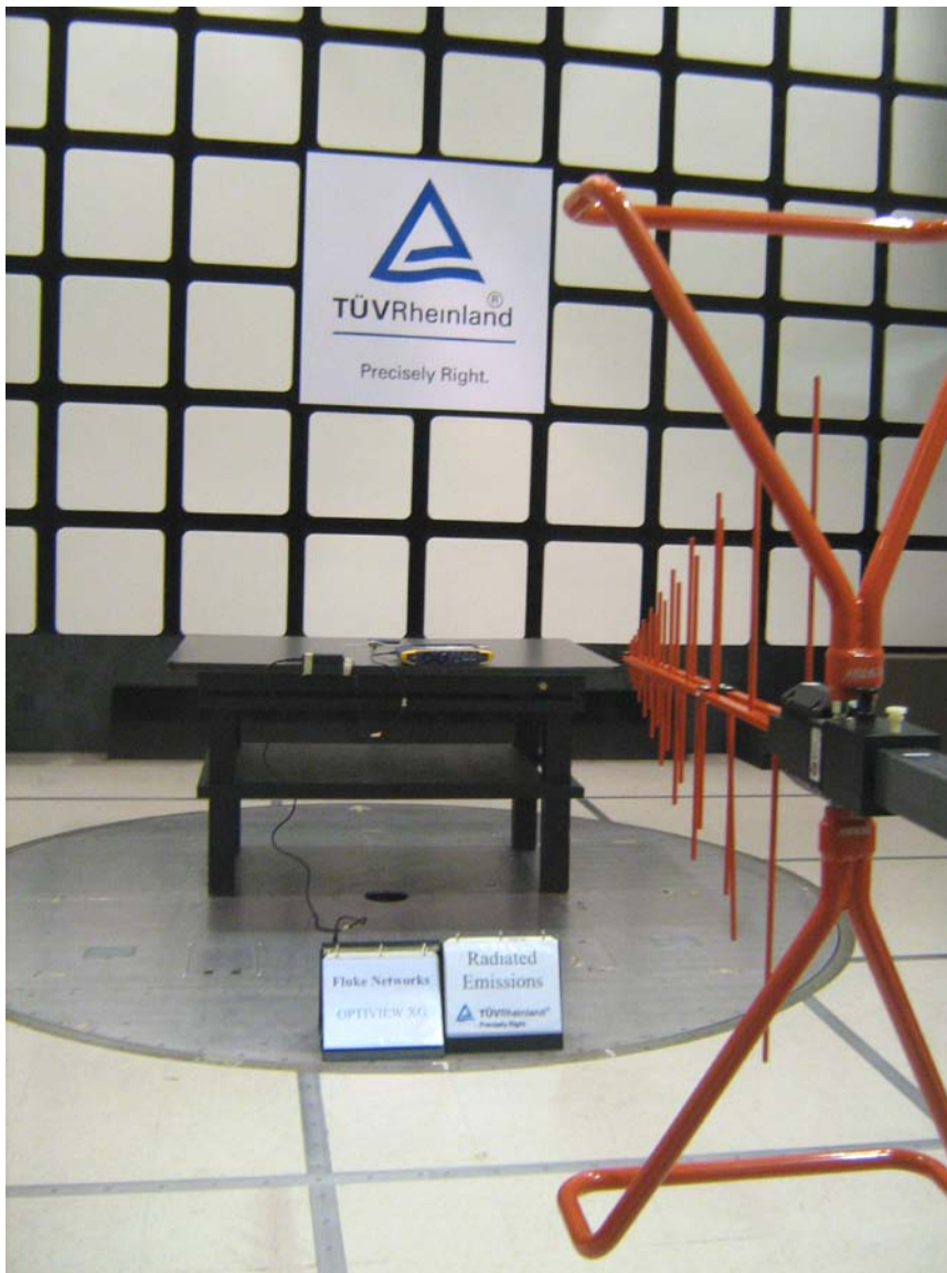
Figure 2: Test Setup for 30 MHz to 1000MHz (Rear View) –OptiView XG on X-Axis
