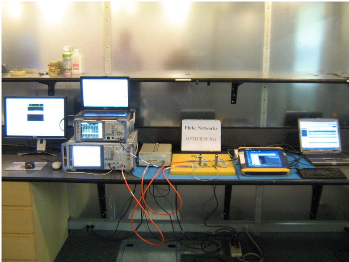
Figure 10: Dynamic Frequency Selection Test Setup
