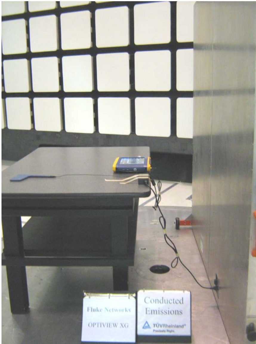
Figure 14: AC Conducted Emission Test Setup (Side View)
