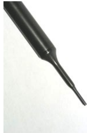
Fig. 5.3 EX3DV3 E-field Probe
