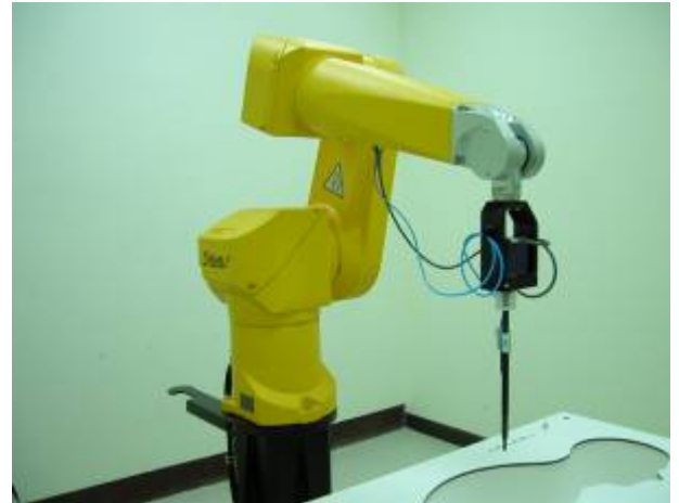
Fig. 5.2 Probe setup on robot
