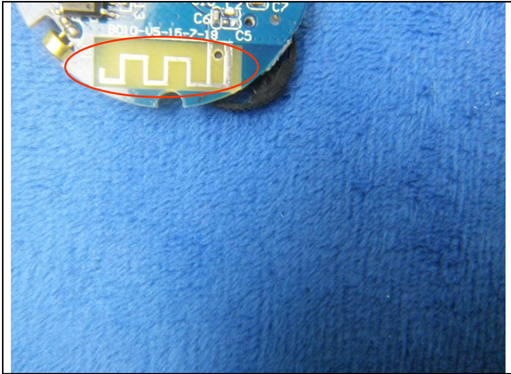
BT - Antenna View
