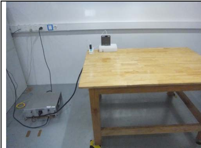
Conducted Emissions Test Setup Front View
