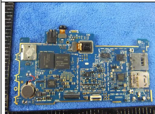
Mainboard without Shielding - Front View
