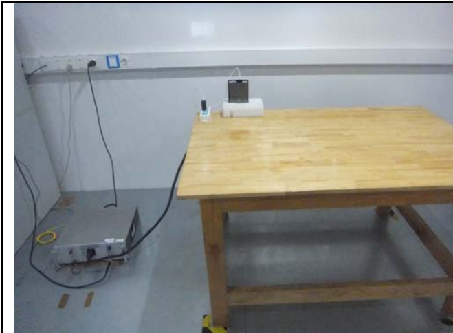
Conducted Emissions Test Setup Front View
