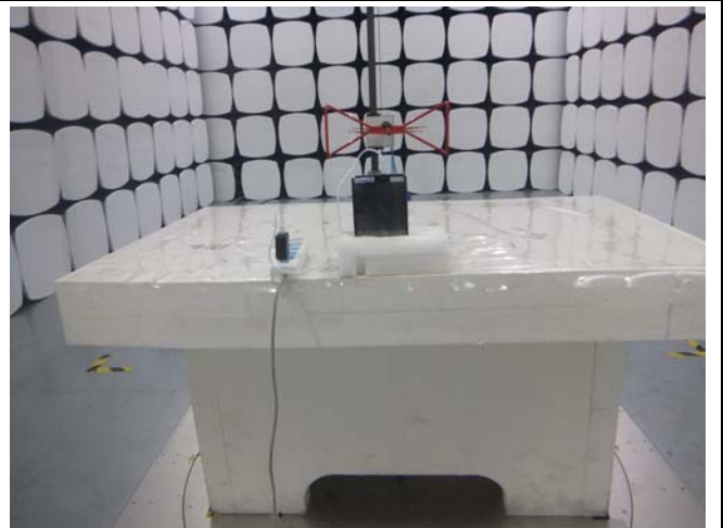
Radiated Spurious Emissions Test Setup Above 1GHz
