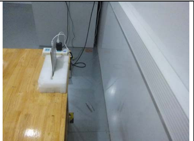
Conducted Emissions Test Setup Side View
