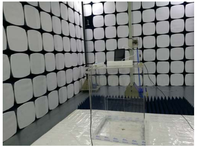
Radiated Spurious Emissions Test Setup Above 1GHz
