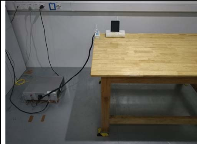
Conducted Emissions Test Setup Front View
