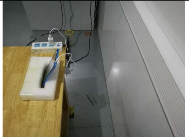
Conducted Emissions Test Setup Side View
