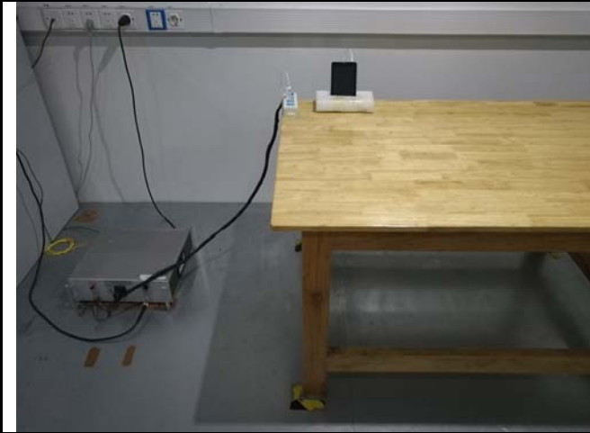
Conducted Emissions Test Setup Front View
