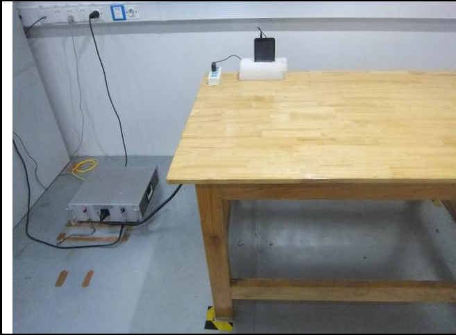
Conducted Emissions Test Setup Front View
