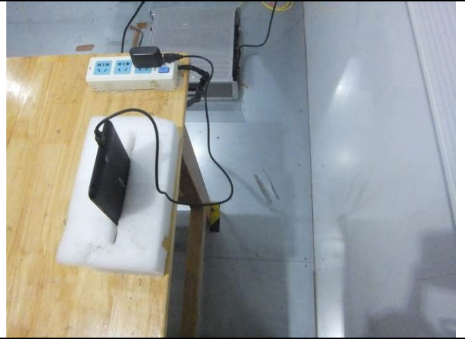
Conducted Emissions Test Setup Side View
