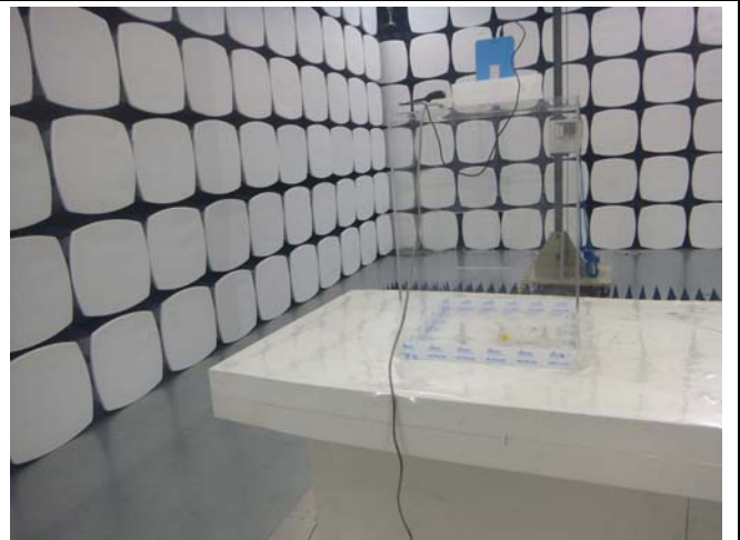
Radiated Spurious Emissions Test Setup Above 1GHz
