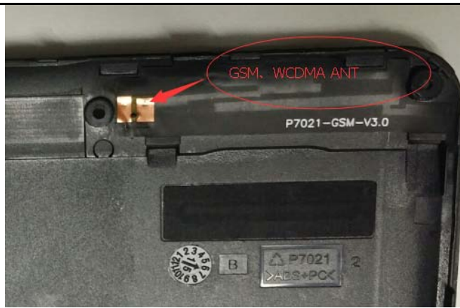
GSM/WCDMA Antenna View
