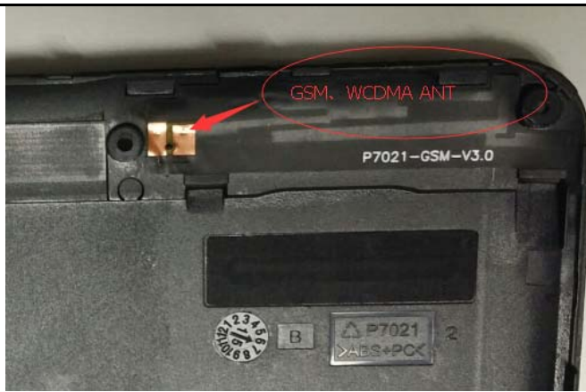
GSM/WCDMA Antenna View
