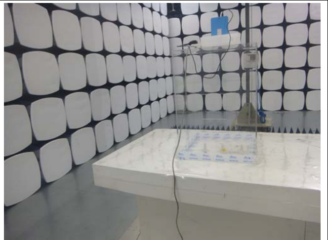
Radiated Spurious Emissions Test Setup Above 1GHz
