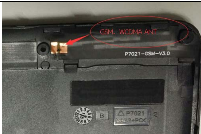
GSM/WCDMA Antenna View
