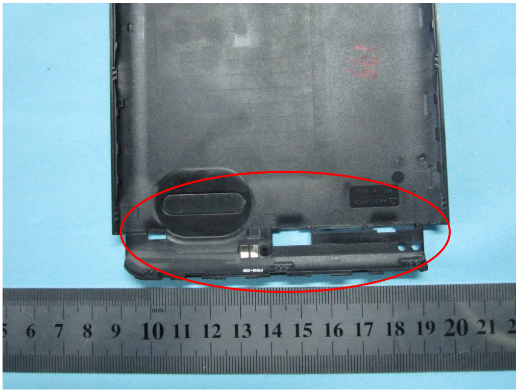
GSM / PCS / UMTS Antenna View
