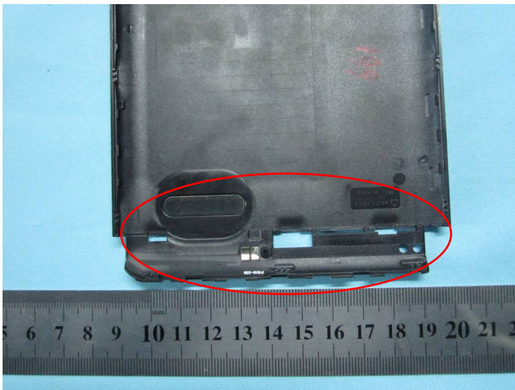
GSM / PCS / UMTS Antenna View
