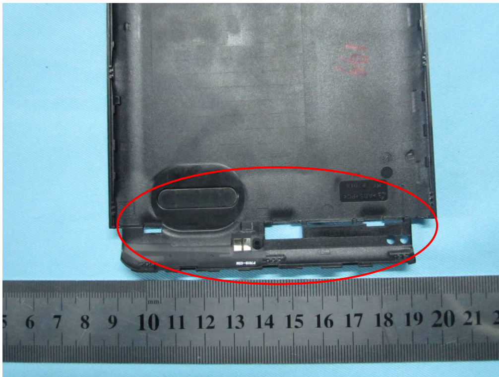
GSM / PCS / UMTS Antenna View
