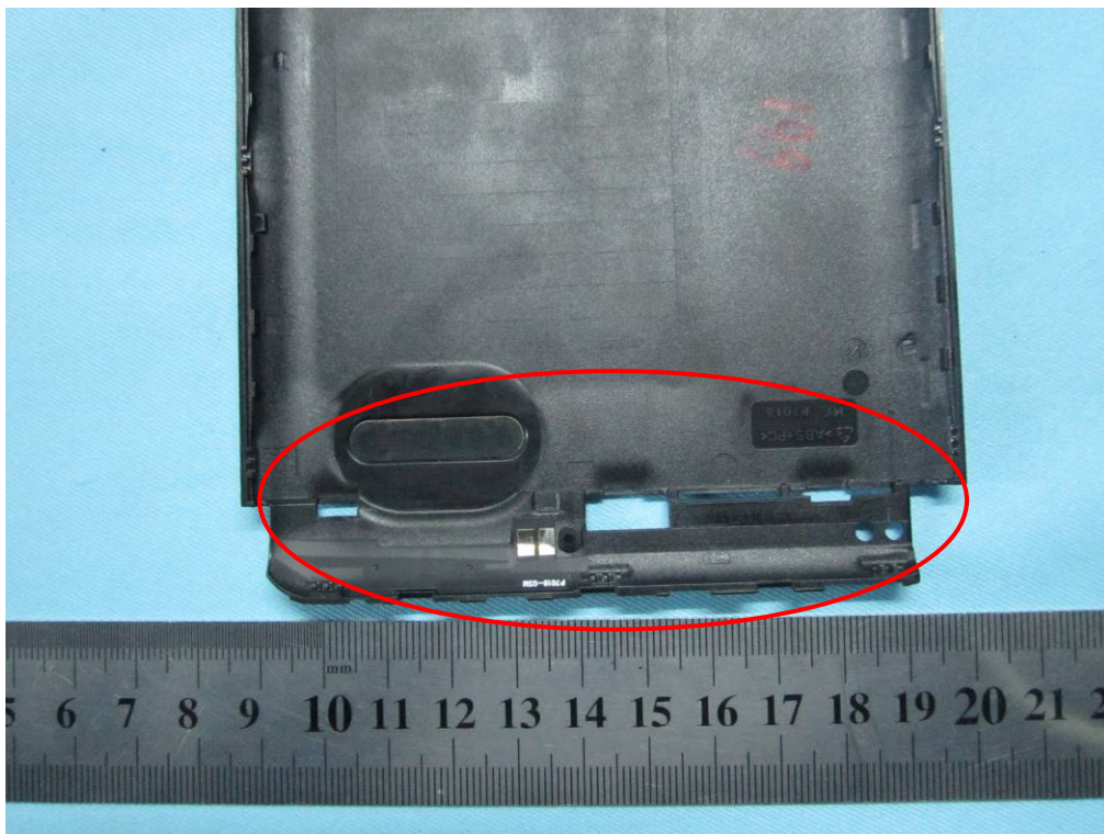
GSM / PCS / UMTS Antenna View
