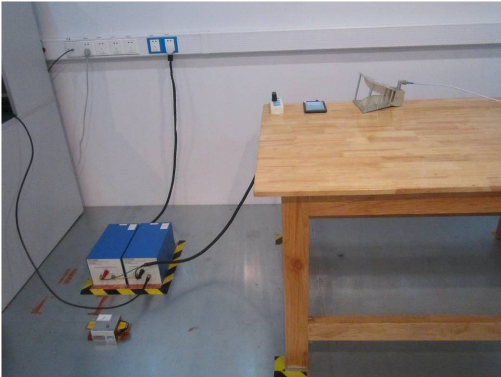
Conducted Emissions Test Setup Front View
