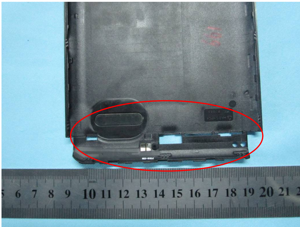
GSM / PCS / UMTS Antenna View
