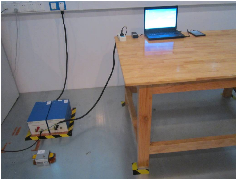
Conducted Emissions Test Setup Front View
