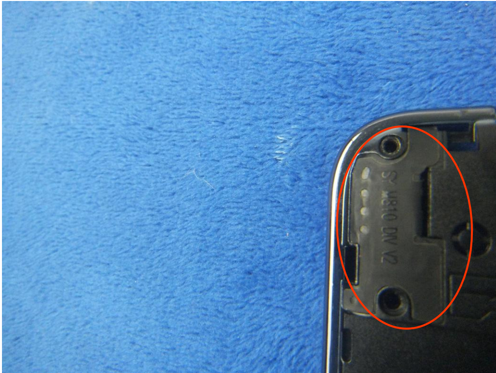
LTE - Antenna View
