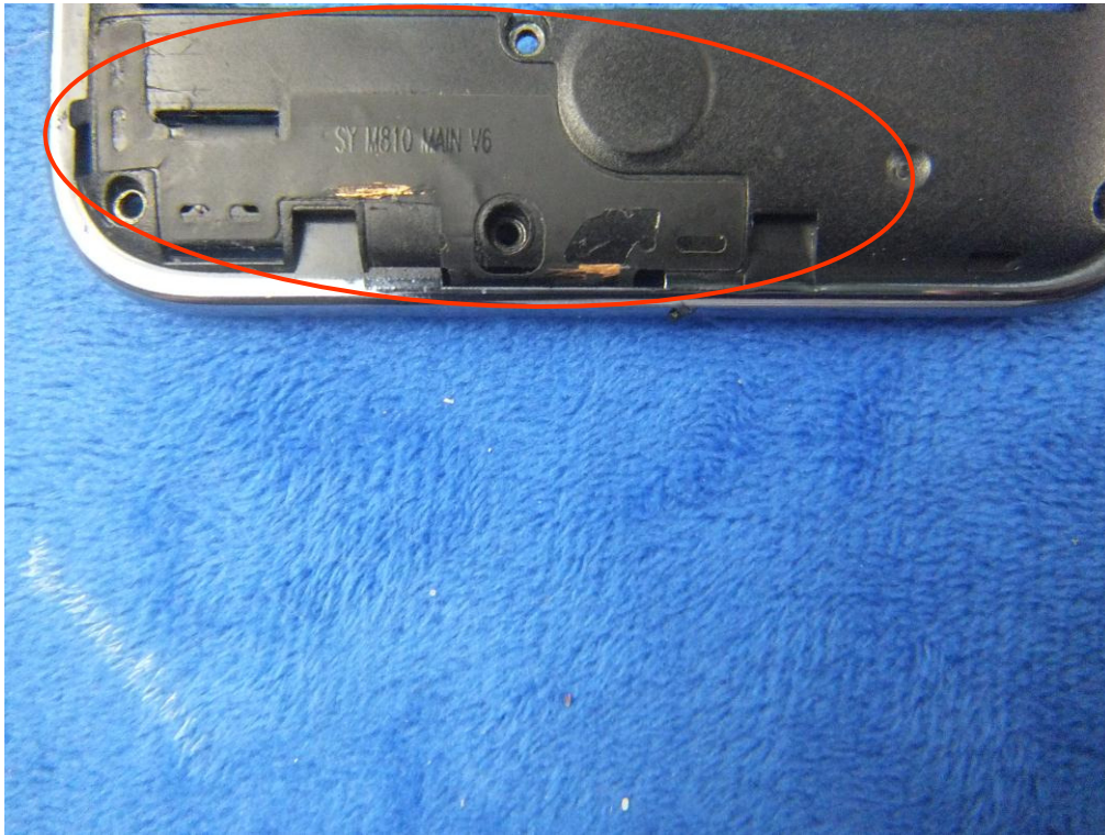
GSM/PCS/UMTS-FDD Antenna View
