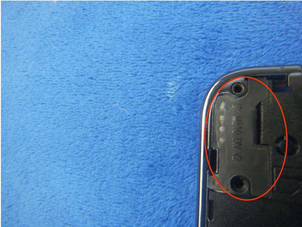
LTE - Antenna View
