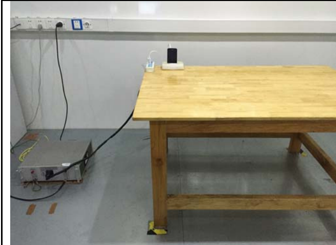
Conducted Emissions Test Setup Front View
