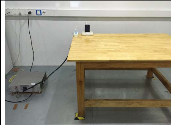
Conducted Emissions Test Setup Front View
