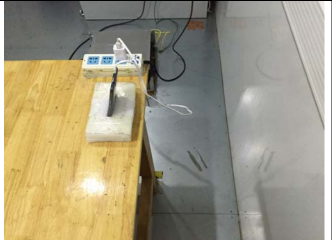
Conducted Emissions Test Setup Side View
