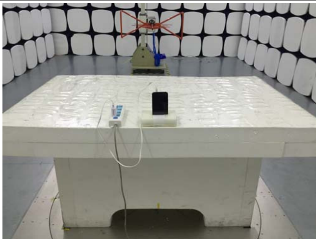
Conducted Emissions Test Setup Front View
