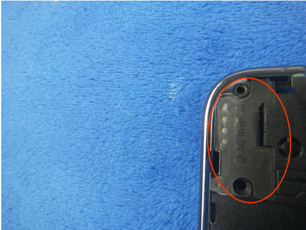
LTE - Antenna View
