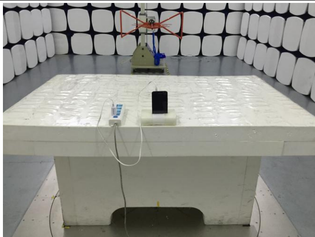
Conducted Emissions Test Setup Front View
