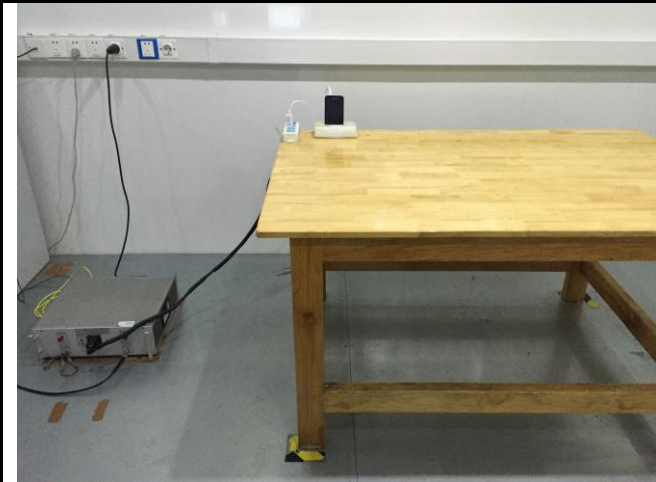
Conducted Emissions Test Setup Front View
