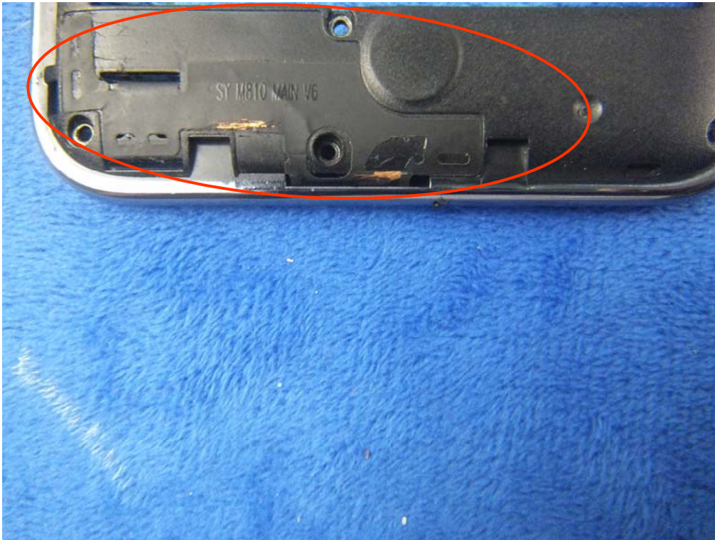
GSM/PCS/UMTS-FDD Antenna View
