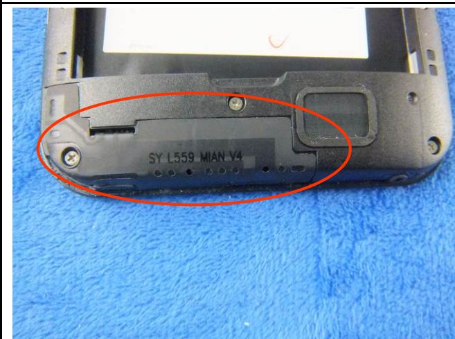
GSM/PCS/UMTS-FDD Antenna View
