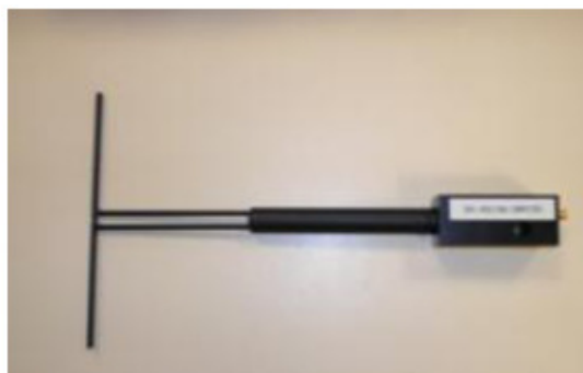
Figure 1 – Satimo COMOSAR Validation Dipole
