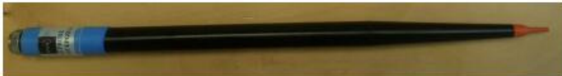
Figure 1 – MVG COMOSAR Dosimetric E field Dipole
