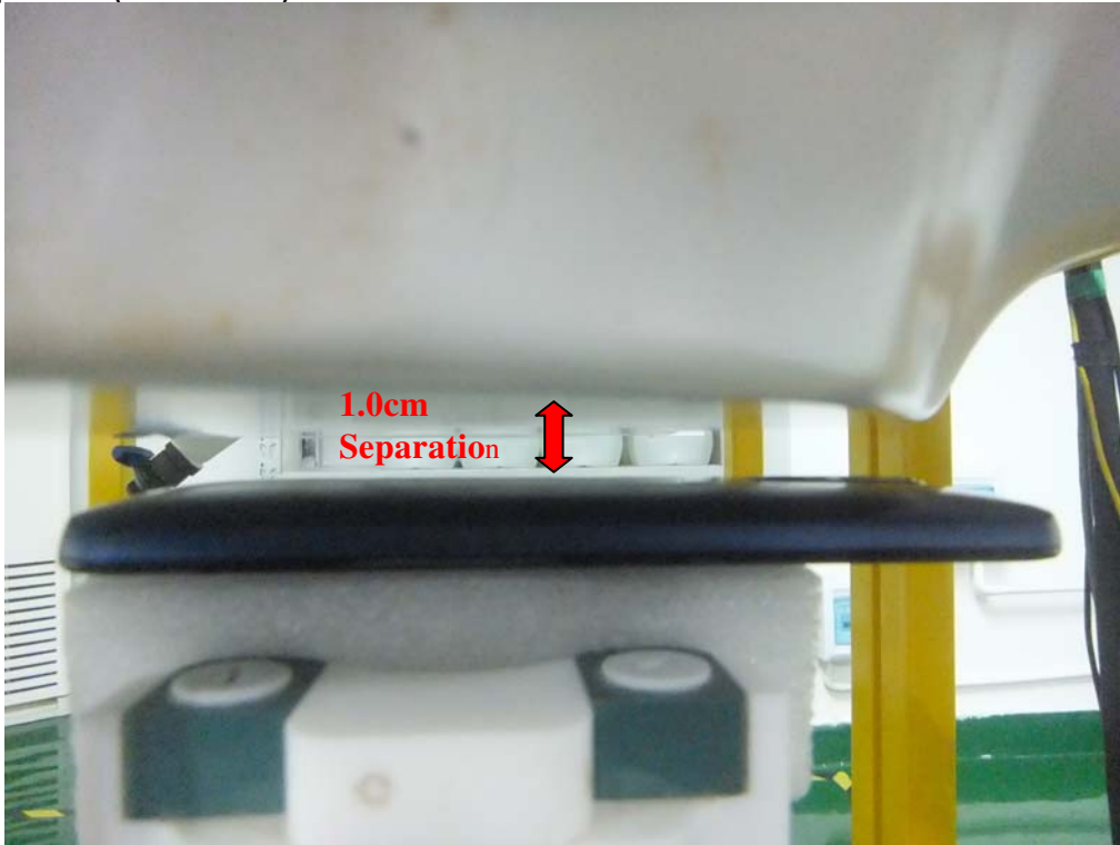
Body Setup Photo (LCD DOWN)
