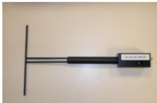
Figure 1 – Satimo COMOSAR Validation Dipole
