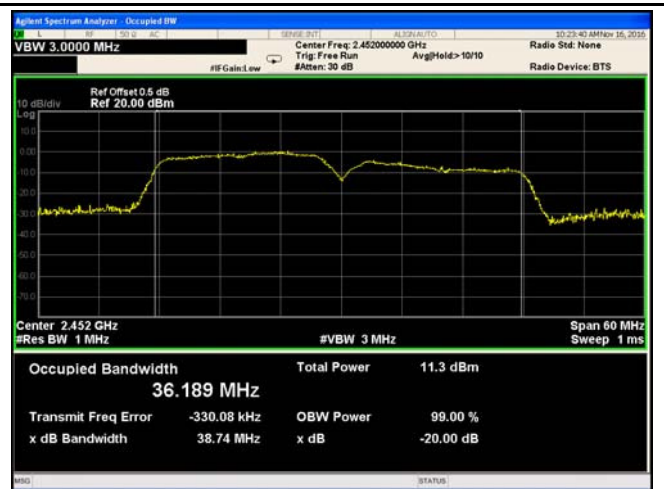
802.11n40 20dB Bandwidth - High CH 2452
