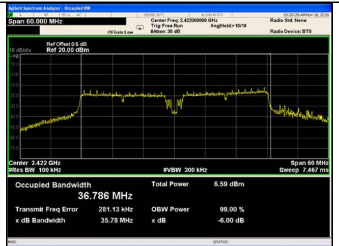
802.11n40 6dB Bandwidth - Low CH 2422
