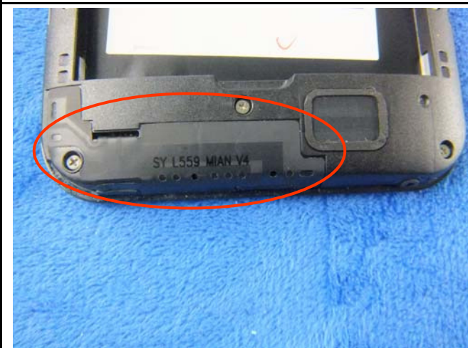
GSM/PCS/UMTS-FDD Antenna View
