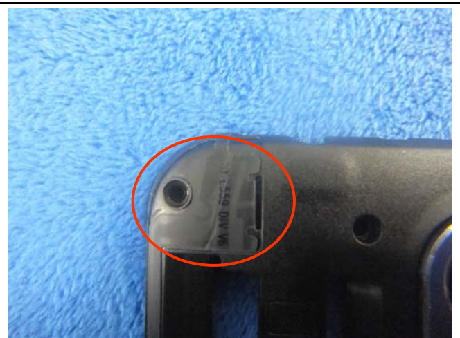
LTE - Antenna View
