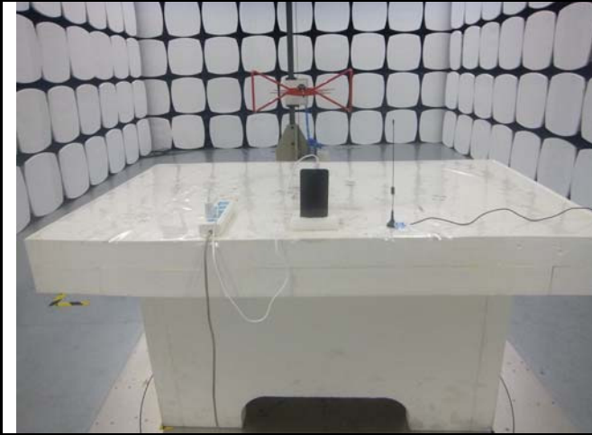
Radiated Spurious Emissions Test Setup Below 1GHz
