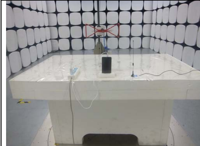
Radiated Spurious Emissions Test Setup Below 1GHz
