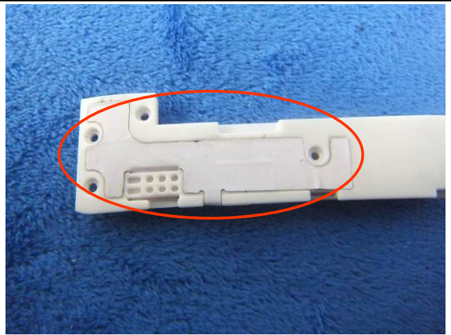
GSM/PCS/UMTS-FDD/LTE Antenna View
