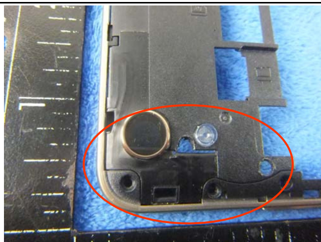
LTE - Antenna View
