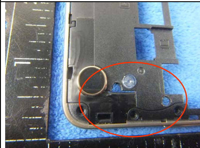
LTE - Antenna View
