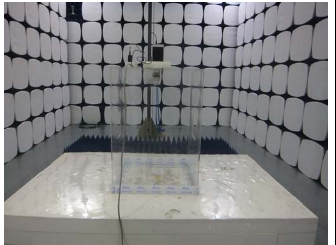
Radiated Spurious Emissions Test Setup Above 1GHz
