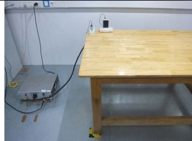
Conducted Emissions Test Setup Front View
