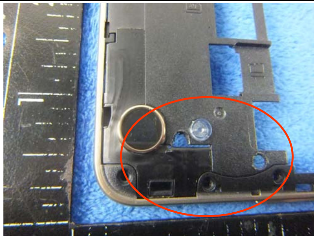
LTE - Antenna View
