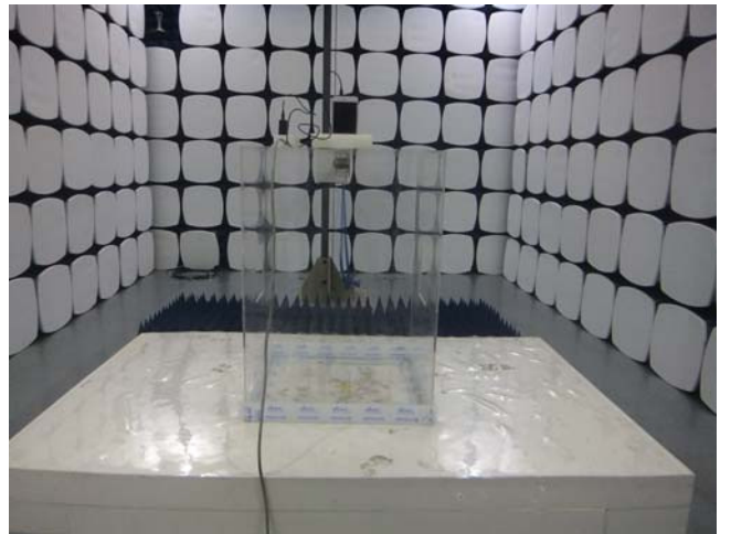
Radiated Spurious Emissions Test Setup Above 1GHz
