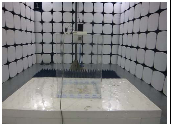
Radiated Spurious Emissions Test Setup Above 1GHz
