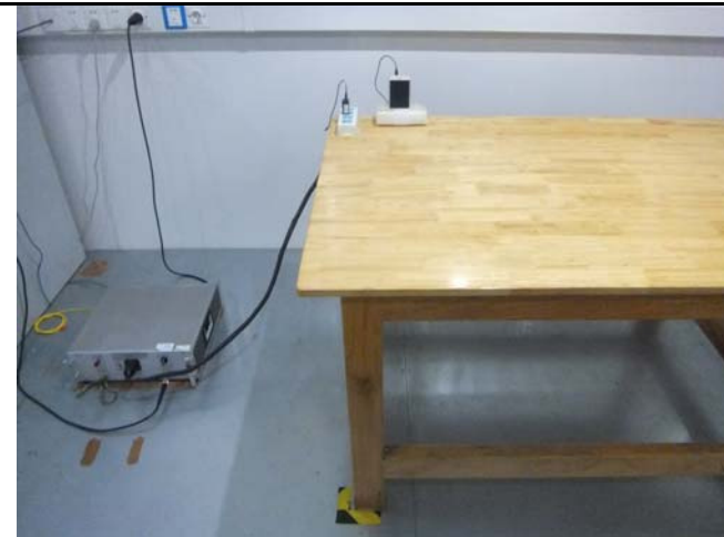
Conducted Emissions Test Setup Front View
