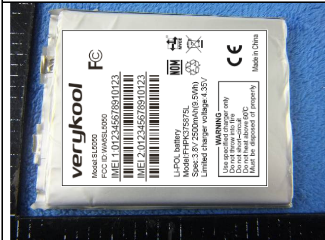
Battery - Front View
