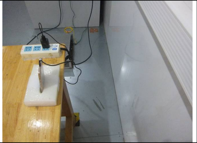
Conducted Emissions Test Setup Side View
